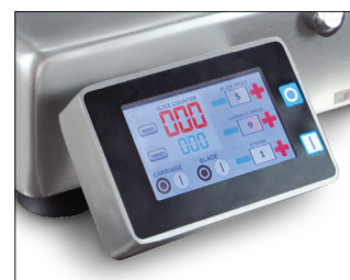
Modern touch panel providing variable blade speed, carriage speed & carriage length.
